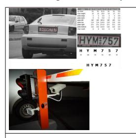
License plate recognition system (optional) scans, detects and performs the character recognition on the license plate number, supported by a camera system, suitable for proper license plate recognition day and night. It automatically forwards the license plate data and pictures for data storage and processing. This way the arrival and exit time of the truck is registered, plus the truck can be called by license plate number.
