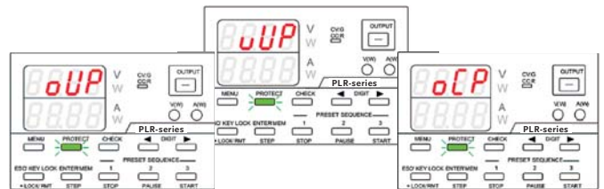
OVP (Over Voltage Protection) UVP (Under Voltage Protection) OCP (Over Current Protection)
