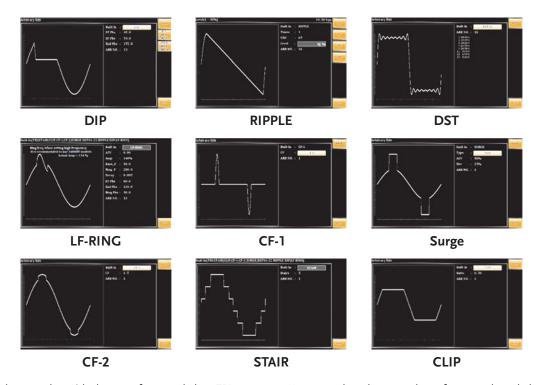
ASR-6000 provides more than 40 built-in waveforms, including: TRI, STAIR, CLIP, CF-1, CF-2, SURGE, DST01-22, RIPPLE, DIP, LF-RING. Each waveform also provides a change setting function, which can modulate thousands of combined waveforms and quickly emulate different AC output environments.
